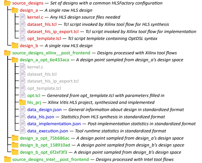
Figure 4. The directory structure that HLSFactory uses. Red are input files; green are the intermediate design points; blue are output files.
